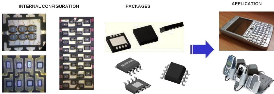
1. Light sensors - These optical devices sense the intensity of light and trigger the automatic switching on and off of headlights and the automatic adjustment of air conditioning settings in cars. The package is a transparent custom-body Quad Flat Pack Leadless Package ("QFN"). The applications of the Light sensors products include Sensor auto switching device, Hall sensor application.
